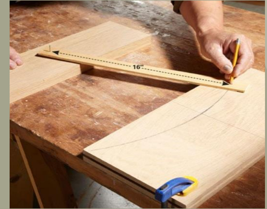
STEP 4: MARK THE ARCH
