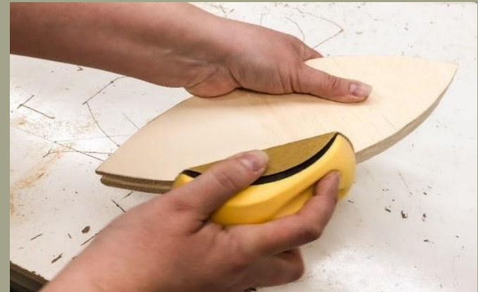
STEP 2 :Stack up the four pieces of each size and sand the edges at the same time. This will keep the shape consistent.
