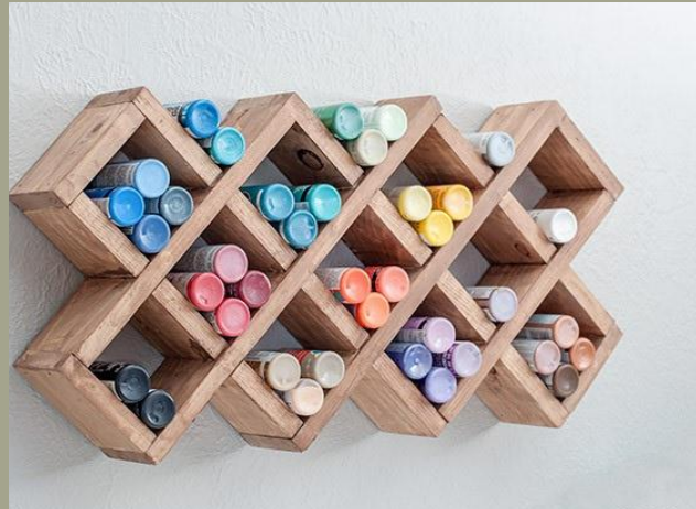
STEP 4: Attach Once you have them all configured and ready, use wood glue and put it together. The end pieces are attached with wood glue and finish nails
